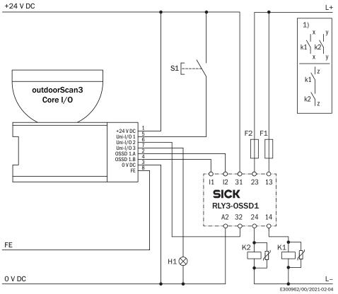
① Output circuits: These contacts must be incorporated into the control such that the dangerous state is brought to an end if the output circuit is open. For categories 4 and 3, they must be incorporated on dual-channels (x, y paths). Single-channel incorporation into the control (z path) is only possible with a single-channel control and taking the risk analysis into account.
