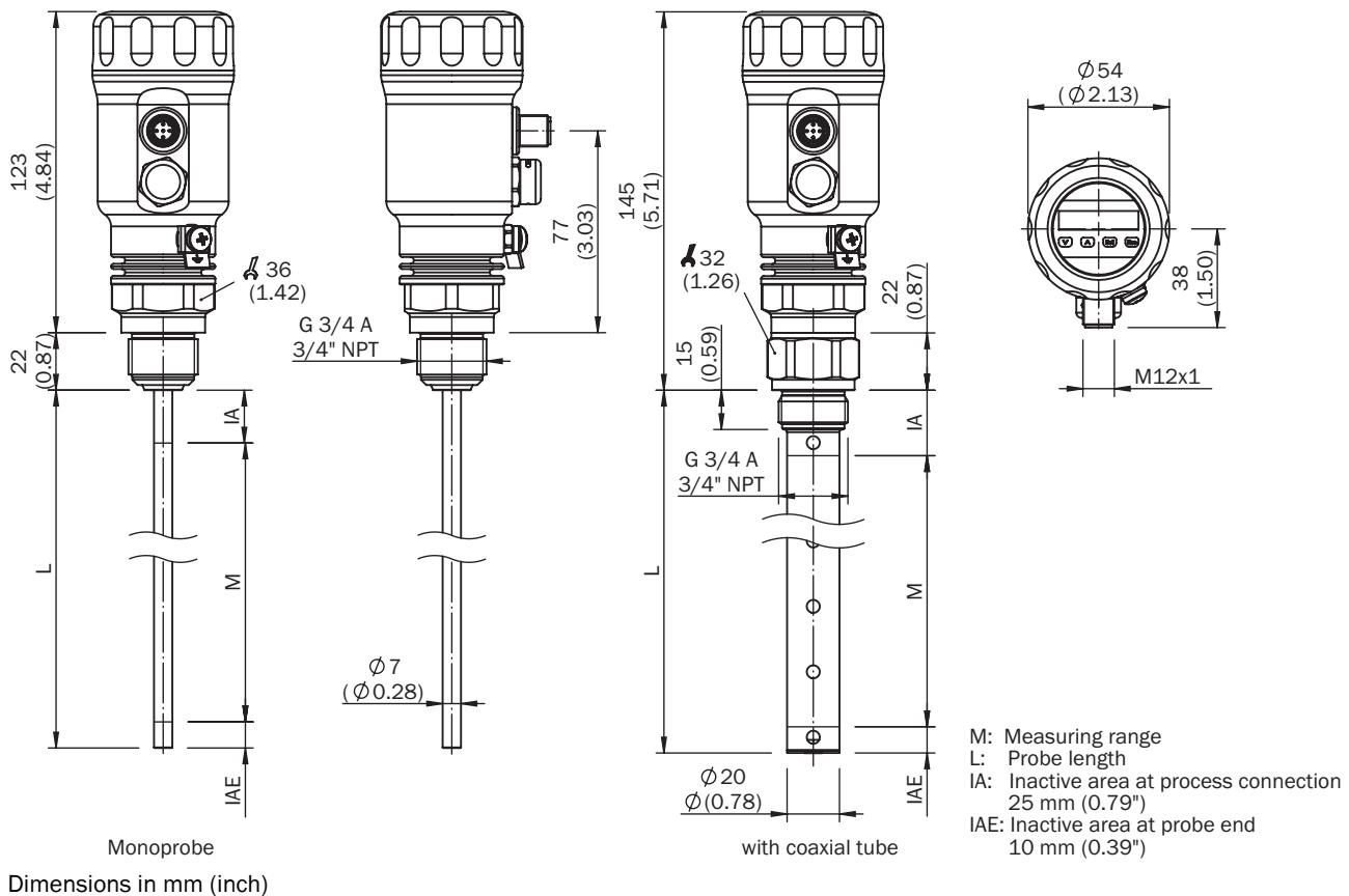
Connection type M12 round connector, 8-pin
