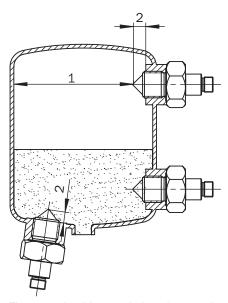
The apex should protrude into the container
