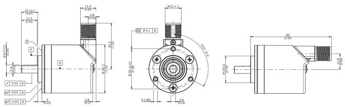
order example for 6 mm shaft diameter: AHx36x-S3xx0xxxxx + BEF-FA-020-036-002 (adapter is not pre-assembled)
