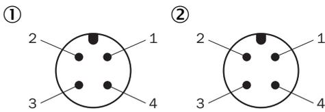
M12 male connector, 4-pin, A-coding
