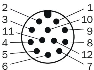
view of M12 male device connector on encoder
