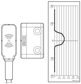
assured switch on distance  $S_{ao}\,6\;mm$
