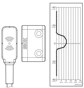
Safe switch on distance  $S_{\text{ao}}\,6~\text{mm}$
