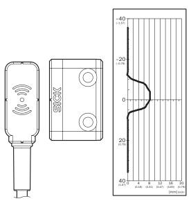
Safe switch on distance  $S_{\text{ao}}\,6~\text{mm}$
