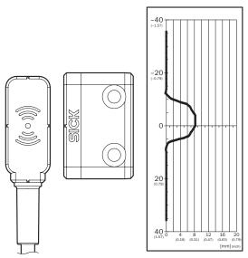
Safe switch on distance  $S_{ao}\,6\;\text{mm}$
