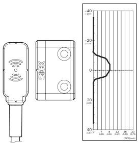
assured switch on distance  $S_{\text{ao}}\,6\,\text{mm}$
