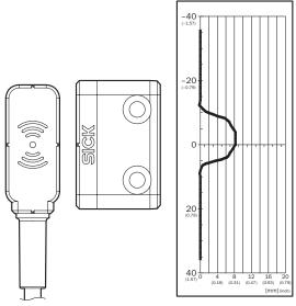
Safe switch on distance  $S_{\text{ao}}\,6\,\text{mm}$
