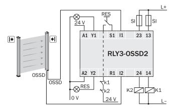
RLY3-OSSD2 at safety light curtain with automated reset and external device monitoring
