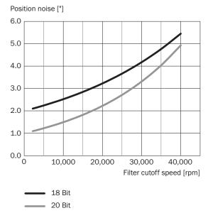
Signal noise is measured as 1 standard deviation ( $\sigma$ ) of the value distribution. Position filter cutoff speed is set by ressource 10Ah, see page 11.
