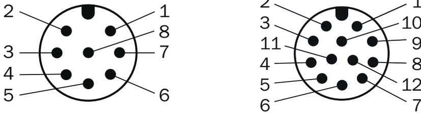
view of M12 male device connector on encoder
