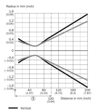
① Minimum distance between sensor and reflector
