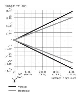
1 Minimum distance between sensor and reflector
