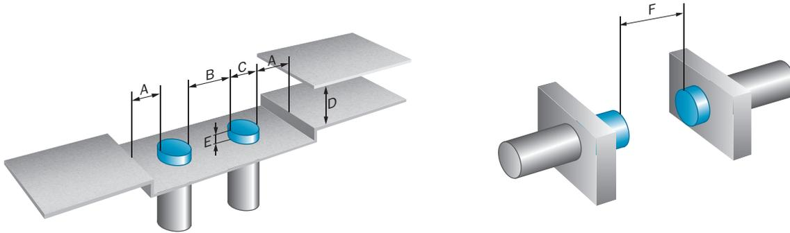
Installation note Flush installation
