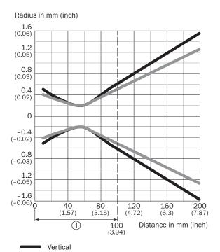
1 Minimum distance between sensor and reflector
