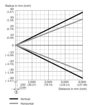
① Minimum distance between sensor and reflector
