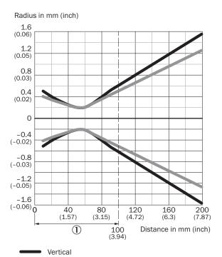
1 Minimum distance between sensor and reflector
