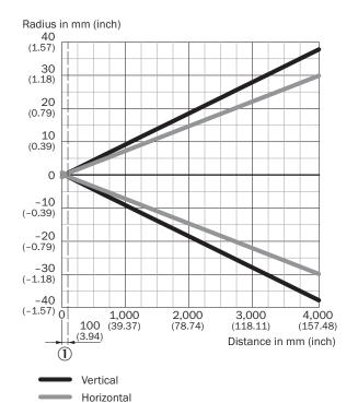
① Minimum distance between sensor and reflector
