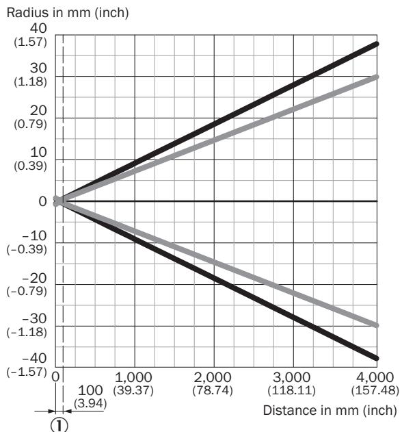
① Minimum distance between sensor and reflector
