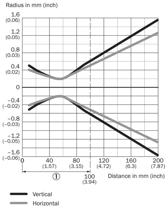
① Minimum distance between sensor and reflector
