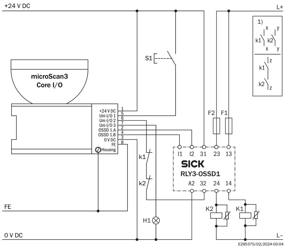
ⓘ Output circuits: These contacts must be incorporated into the control such that the dangerous state is brought to an end if the output circuit is open. For categories 4 and 3, they must be incorporated on dual-channels (x, y paths). Single-channel incorporation into the control (z path) is only possible with a single-channel control and taking the risk analysis into account.
