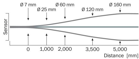
Sensing range diagram WL4S-3, WLG4S-3, 5 m
