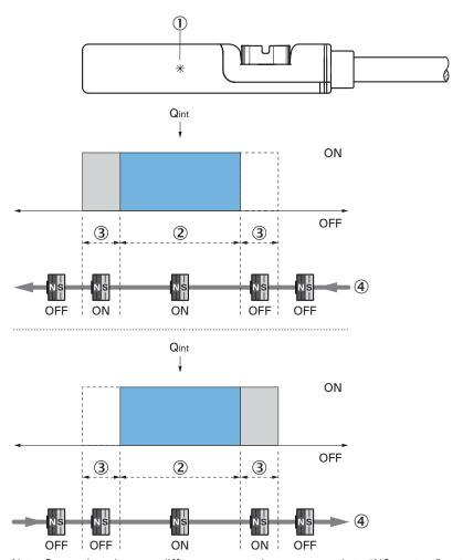
Note: Sensor housing may differ; representation corresponds to "NO contact" output function; overrun distance = switching point width + hysteresis
