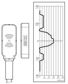
Assured switch on distance Sao 9 mm. Observe border areas for parallel approach: a minimum distance of 4 mm (typical) must be upheld when the actuator moves laterally to the sensor surface. This prevents early triggering due to the side preparation areas.
