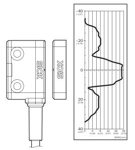
Assured switch on distance Sao 14 mm. Observe border areas for parallel approach: a minimum distance of 10 mm (typical) must be upheld when the actuator moves laterally to the sensor surface. This prevents early triggering due to the side preparation areas.
