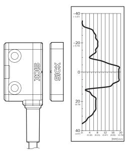
Assured switch on distance Sao 14 mm. Observe border areas for parallel approach: a minimum distance of 10 mm (typical) must be upheld when the actuator moves laterally to the sensor surface. This prevents early triggering due to the side preparation areas.
