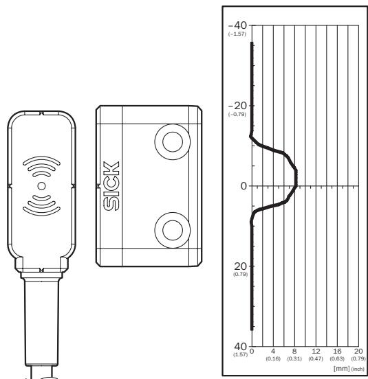
assured switch on distance  $S_{ao}$  6 mm
