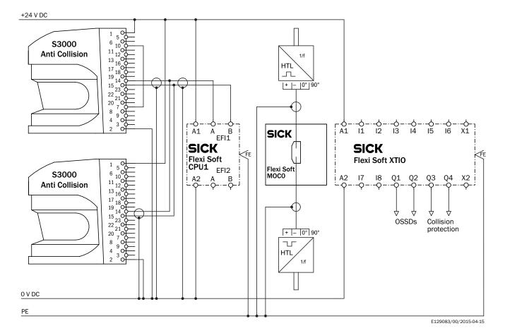
Host-Guest network with two S3000 Anti Collision and Flexi Soft modular safety controller
