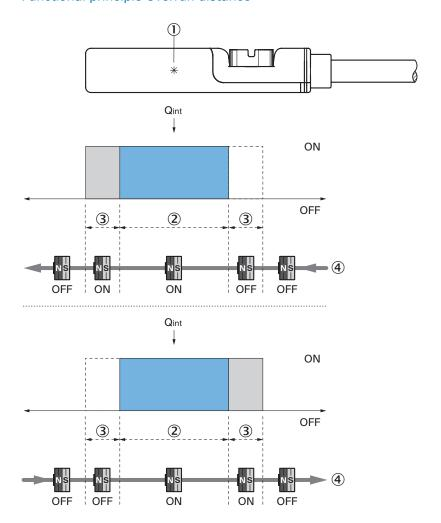
Note: Sensor housing may differ; representation corresponds to "NO contact" output function; overrun distance = switching point width + hysteresis
