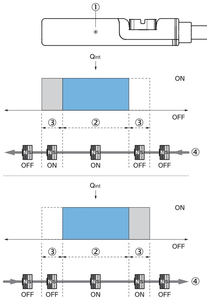
Note: Sensor housing may differ; representation corresponds to "NO contact" output function; overrun distance = switching point width + hysteresis
