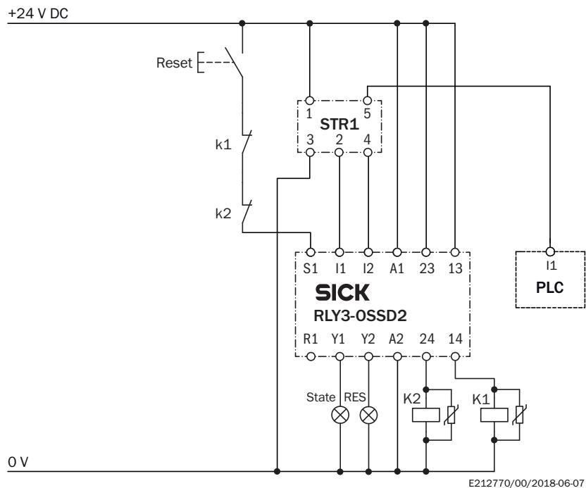
Connection diagram Parallel connection of two STR1 RFID safety switches to a Flexi Classic safety controller
