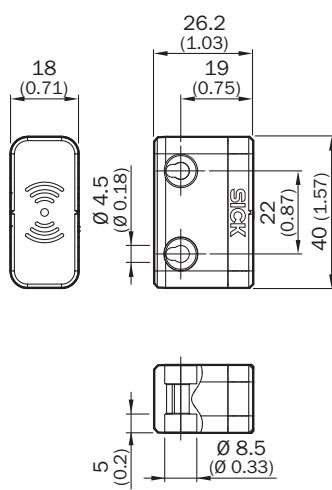
Response range "Standard" actuator, active front sensor surface
