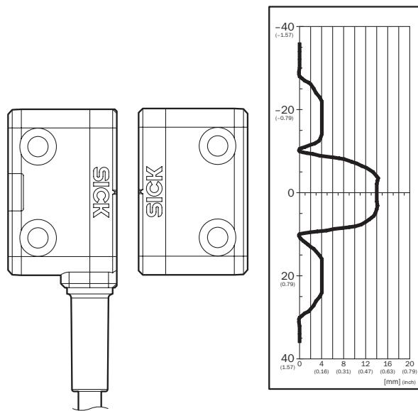
Assured switch on distance  $S_{ao}$  10 mm. Observe border areas for parallel approach: a minimum distance of 6 mm (typical) must be upheld when the actuator moves laterally to the sensor surface. This prevents early triggering due to the side preparation areas.
