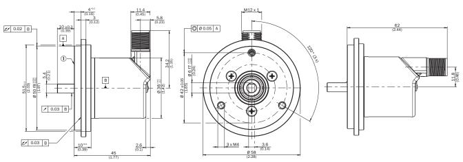
order example for 6 mm shaft diameter: AHx36x-S3xx0xxxxx + BEF-FA-020-050 (adapter is not pre-assembled) (1) Measuring point for operating temperature
