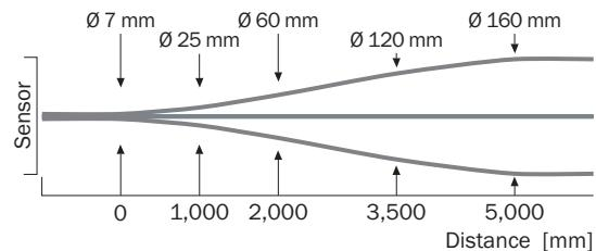
Sensing range diagram WL4S-3, WLG4S-3, 5 m
