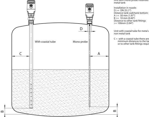
Unit with mono probe mounted in metal tank
