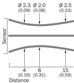
Sensing range diagram GTB2S, 15 mm
