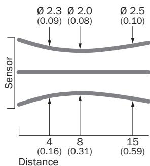
Sensing range diagram GTB2S, 15 mm
