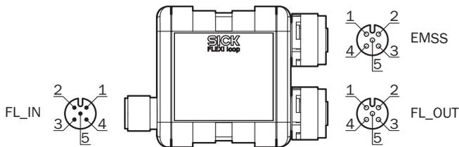
The FL\_IN pin assignment is only relevant for the first loop node in a safe series connection when connected to Flexi Soft. Additional Flexi Loop nodes are connected to FL\_OUT using standardized cables with M12 plug connectors.
