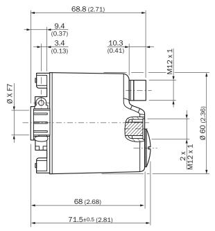
Dimensions in mm (inch) diameter x f7 corresponds to the shaft diameter
