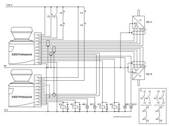
S300 Professional with S300 Professional in host/guest connection with relays/contactors Operating mode: with restart interlock and external device monitoring
