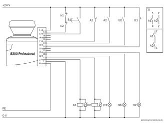
S300 Professional in connection with relays/contactors Operating mode: With restart interlock and external device monitoring Protective field switching with control inputs IN A and IN B Comments
