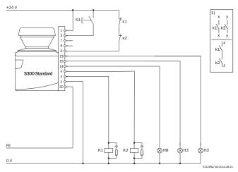
S300 Standard in conjunction with relays/contactors
