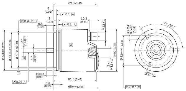
Dimensions in mm (inch) diameter x f7 corresponds to the shaft diameter
