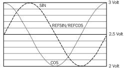
Signal diagram for clockwise rotation of the shaft looking in direction "A" (see dimensional drawing) 1 period =  $360^{\circ}$ :  $1024^{\circ}$
