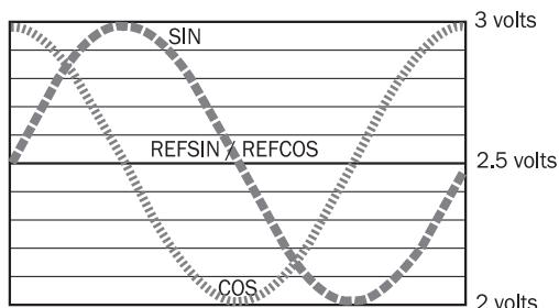
Diagrams Signal specification of the process channel
