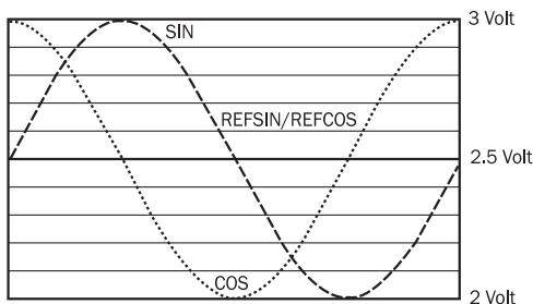
Signal diagram for clockwise rotation of the shaft looking in direction "A" (see dimensional drawing)
