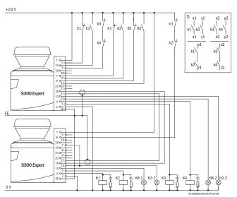
S300 Expert with S300 Expert in host/guest connection with relays/contactors Operating mode: with external device monitoring and without restart interlock Static protective field switching using the control inputs A, B and C The protective fields affect the related OSSDs on host or guest **Comments**
