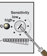
If yellow LED illuminates, turn "Sensitivity" rotary switch counter-clockwise until the yellow LED just goes out.
