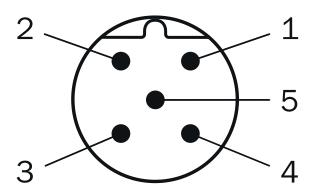
Male connector M12, 5-pin, A-coded
