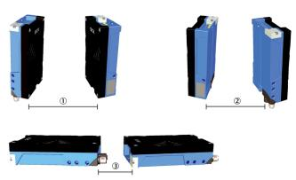
Distances required to prevent mutual interference with mounting of two devices.
